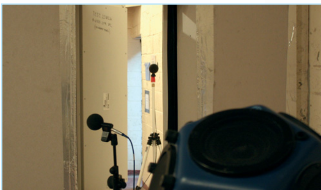
Profab access panel undergoing acoustic testing
